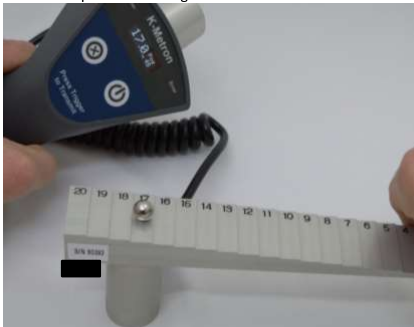
19mm Sphere Validating Calibration – use the provided +10mm disk to measure units over 20mm.
